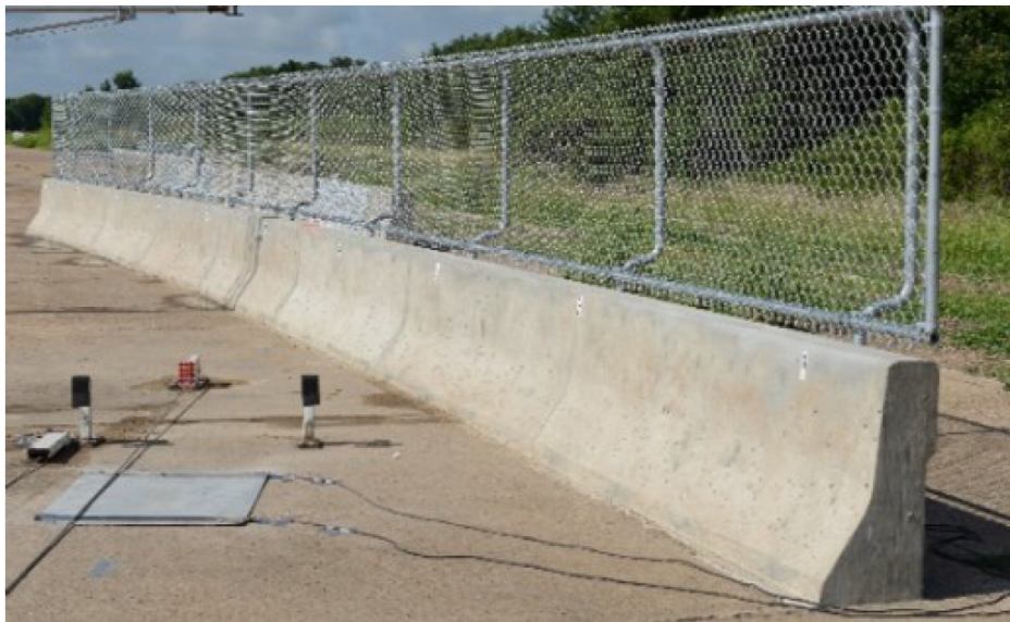
Figure 3.42 : Tested retrofitted design on the test site
