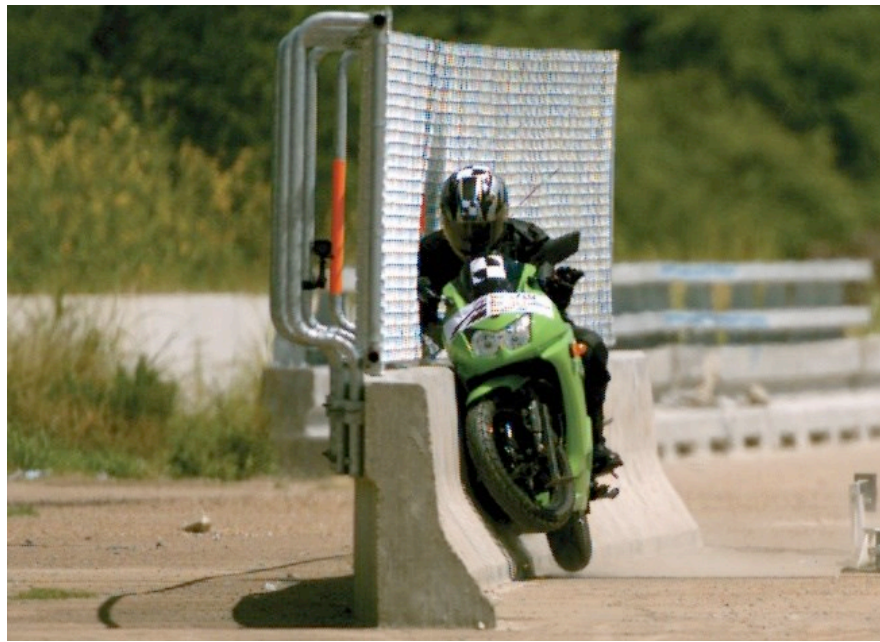
Figure 3.43 : Motorcycle and dummy impacting the concrete and chain fence barrier during the crash test; Source: Texas A&M Transportation Institute
