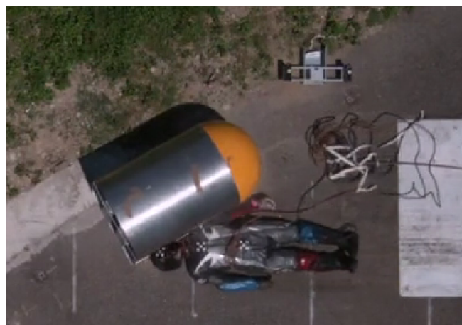
Figure 3.7 : Testing of the Armadillo crash cushion according to CEN/TS 17342:2019 Standard
