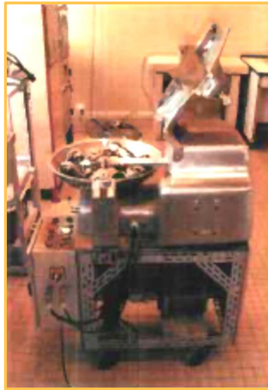
Picture 32: Disintegrating mixer - Detail of the mixer (GTS)
