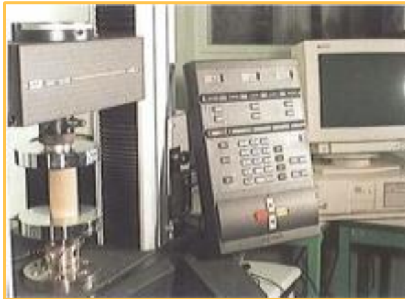
Picture 30: Measurement of the unconfined compressive strength
