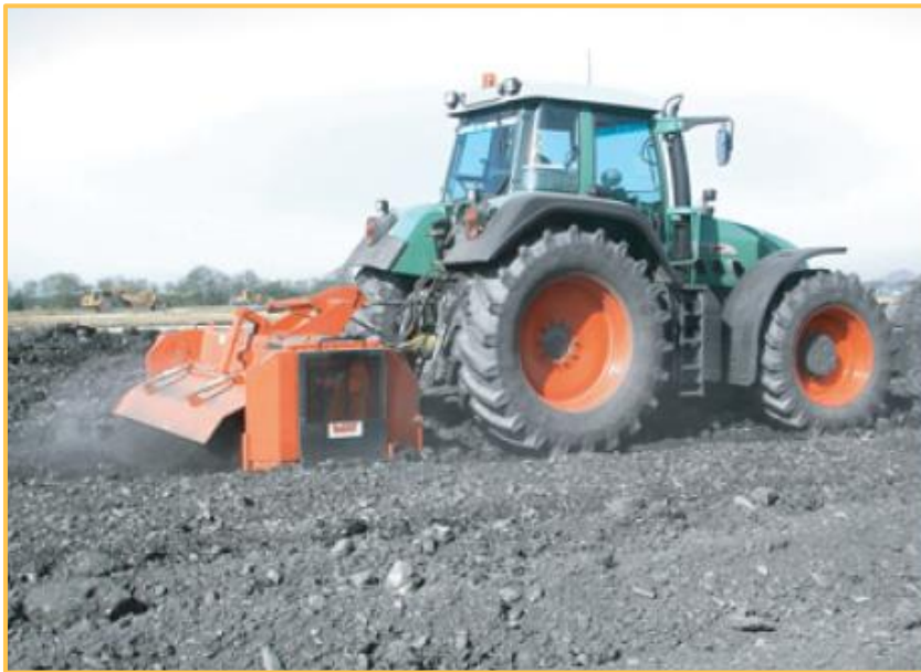
Picture 9: Stone crusher on a tractor (RAZEL)
