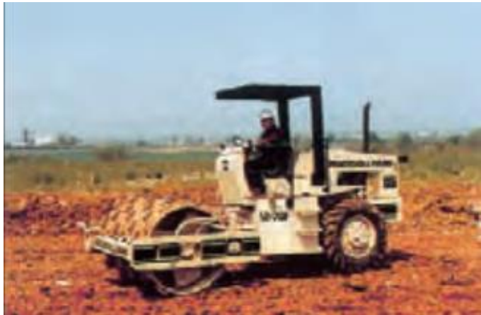
Picture 21: Vibrating compactors (Photos GTR)
