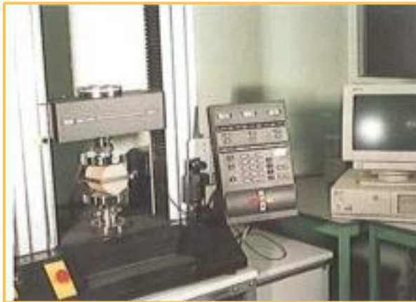
Picture 31: Measurement of the diametral compressive strength
