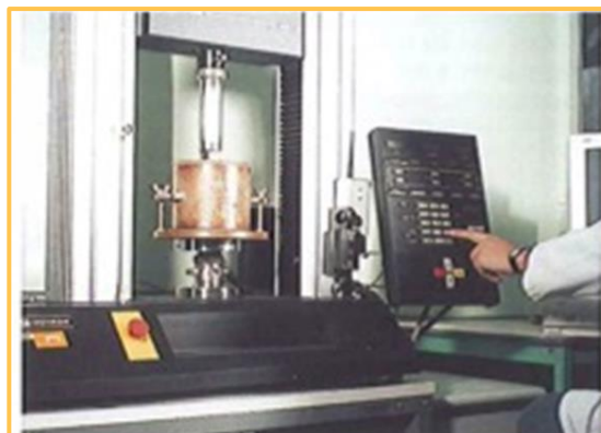
Picture 24: IPI test (similar to Immediate CBR test but without surcharge)
