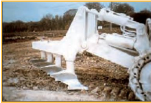
Detail of mixing action produced by blades ploughs
