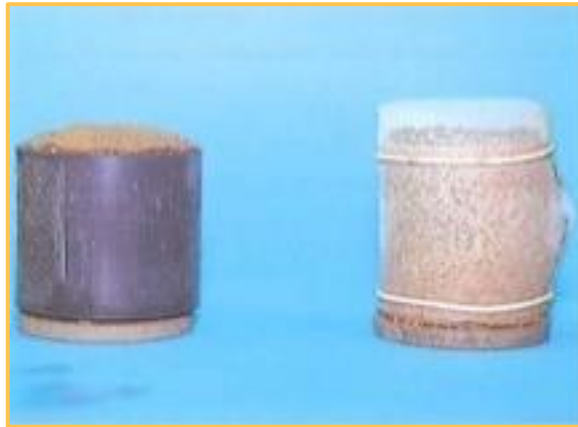
Picture 28: Test to assess suitability of a soil for treatment with lime and/or hydraulic binder (detail)
