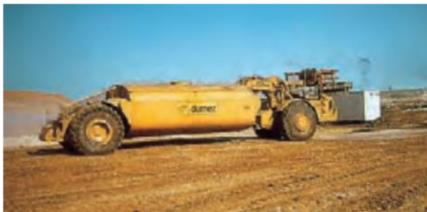
Carp tail sprinkler / large capacity tank on a scraper (photo GTR & GTS)
