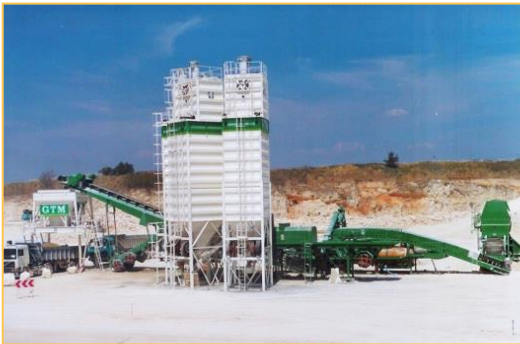
Motorway A837 France Hydraulic binder treatment plant / Crushed soft limestone 0/60 mm (Photos GTM Terrassement)
