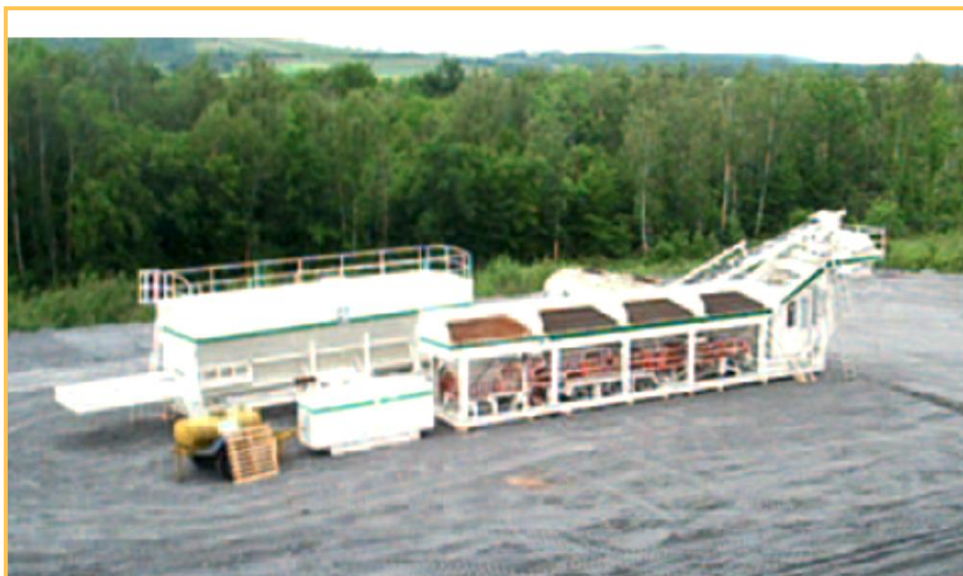
Picture 18: Mixing plant / Treatment of fly ash with binders for capping layer (Photo Techniques de l'Ingénieur)
