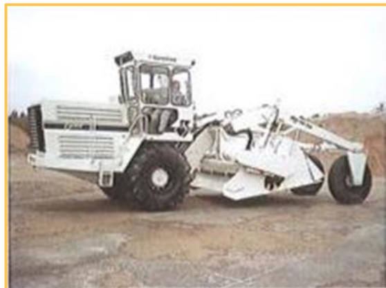
Second generation soil pulveriser with mixing chamber between front and rear axles, maximum mixed layer thickness 0.35m (after compaction).
