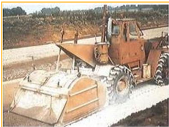
First generation soil pulveriser with mixing chamber at rear of tractor, maximum mixed layer thickness 0.3m (after compaction).
