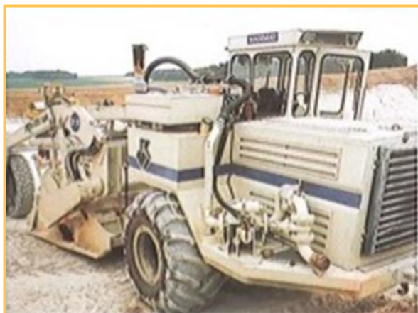
Picture 44: Capping layer Job site / Device for injecting water into the mixing chamber
