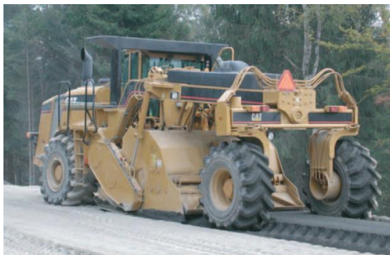
Picture 16: Pulvimixers of different types
