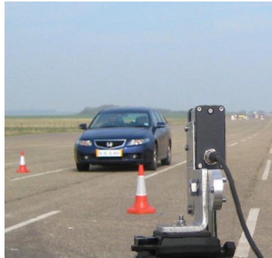
Figure 4.5: Single laser beam systems applicable to a wide variety of traffic control and law enforcement scenarios. The photo illustrates the CMP52 laser radar developed by Noptel Oy (Noptel Oy, 2021).
