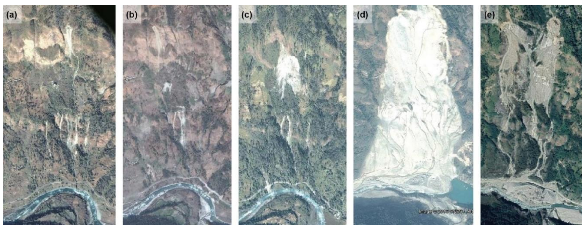
Fig 6.1 Progressive development of the Jure landslide on the Arniko Highway, Nepal. (a) Nov 2000; (b) Aug 2004; (c) Oct 2012; (d) Dec 2014; (e) Nov 2020. From Hearn 2021 , reproduced with permission of the Geological Society, London
