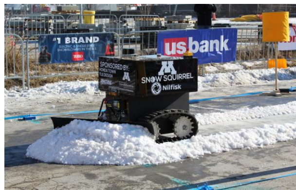
Figure B.32: AI-powered autonomous snowploughs use sensors, ML, and real-time data to map, detect obstacles, and optimise clearing, improving winter road safety (University of Minnesota Robotics, 2024).
