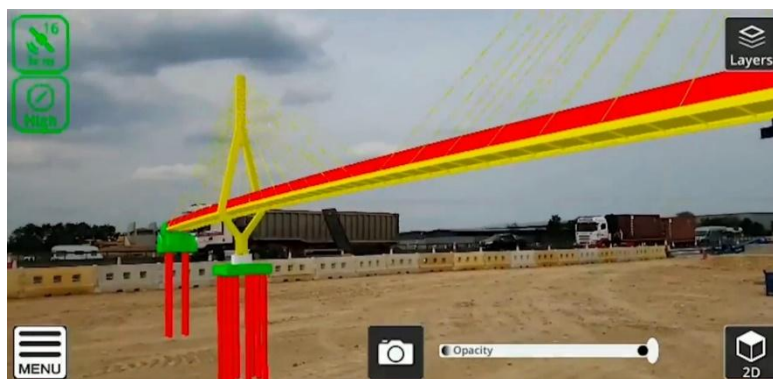
Figure B.12: GNSS-integrated AR enhances spatial awareness and precision in road design, as shown in the A14 Cambridge to Huntingdon project with Trimble SiteVision (Trimble SiteVision GNSS, 2024).
