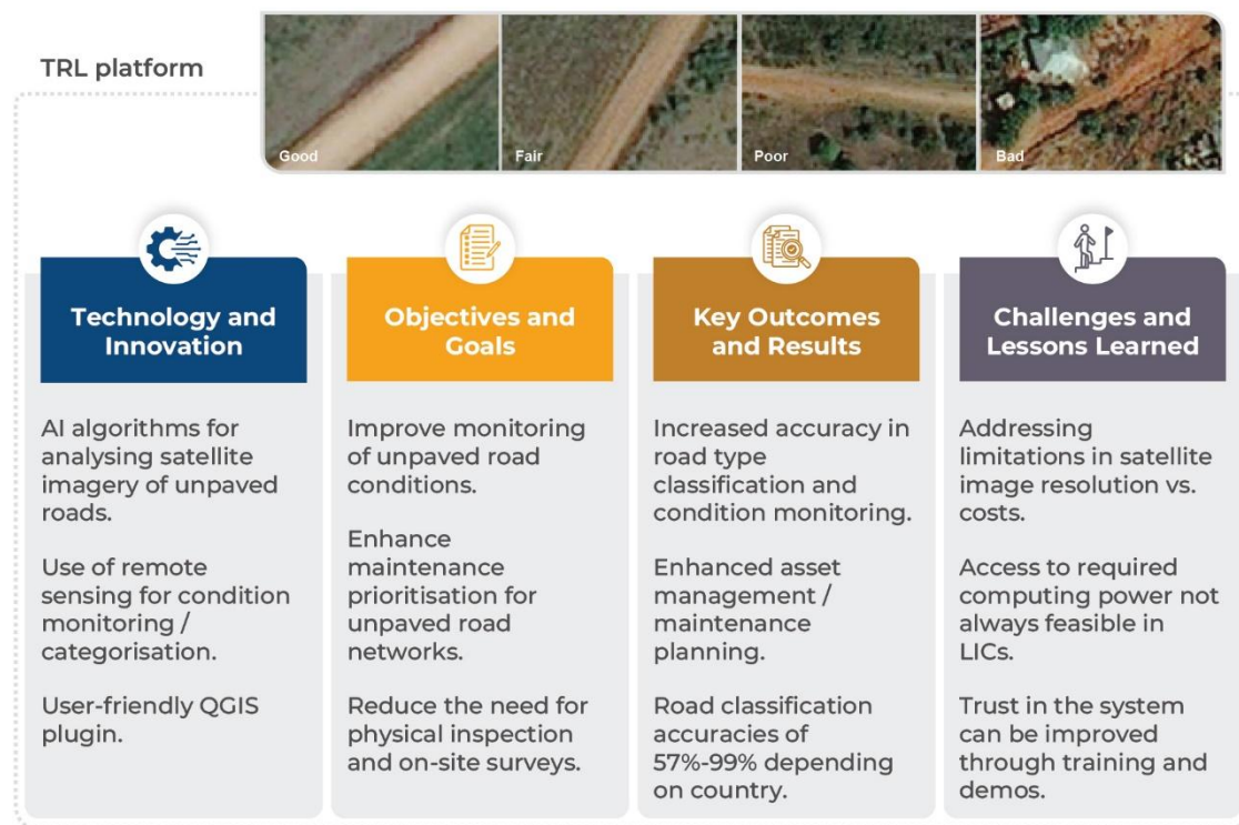
Figure 5.6: TRL - Monitoring of unpaved road conditions in Africa using satellite imagery and AI.
