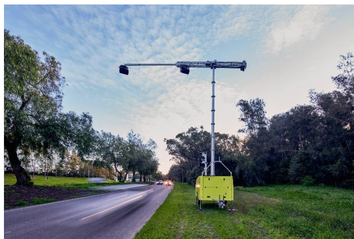
Figure E.11: Mobile camera for enforcement of mobile phone and seatbelt offences (Acusensus, 2024)
