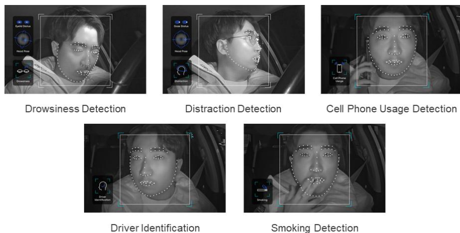
Figure B.39: AI enhances vehicle safety by monitoring driver behaviour in real time, detecting drowsiness, distraction, phone use, and smoking, issuing alerts to prevent crashes (Nota AI, 2024; Zhao et al., 2020).
