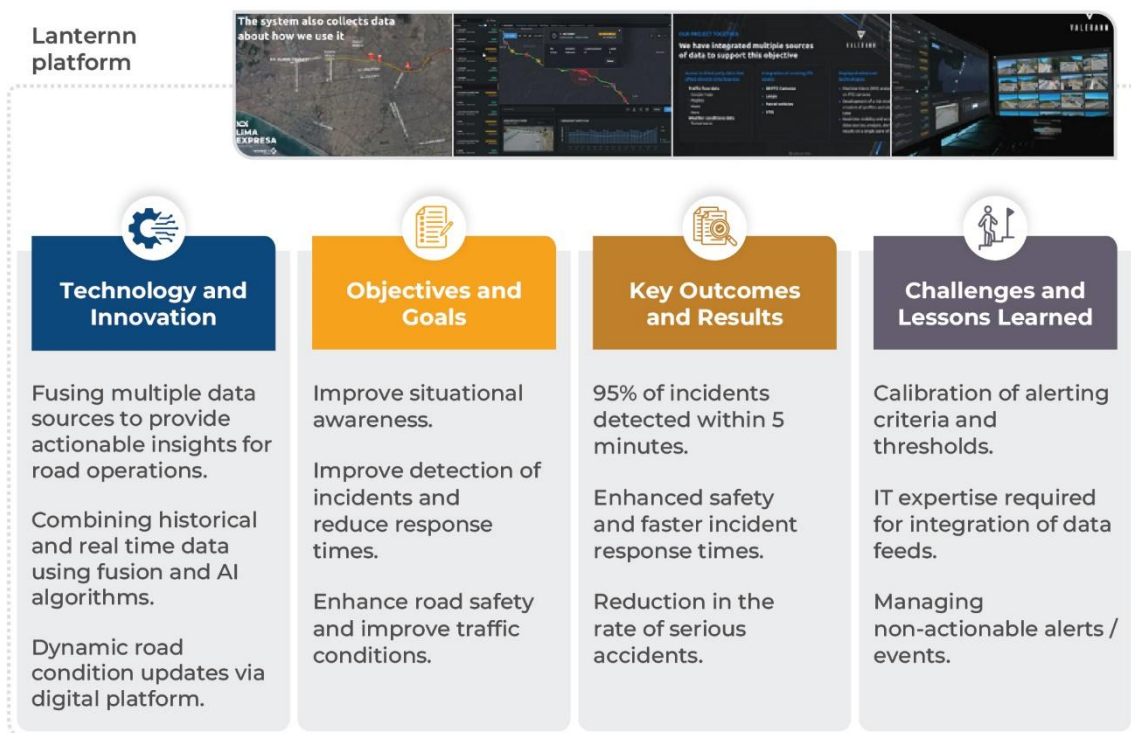
Figure 5.3: Lanternn by Valerann used for incident detection in Lima, Peru.
