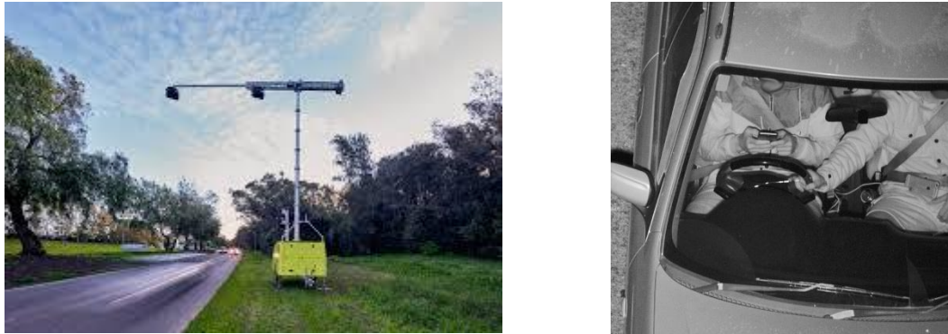
Figure B.38: AI-powered cameras monitor vehicle interiors to detect mobile phone use and seatbelt violations, enhancing safety through compliance enforcement (Acusensus, 2024).
