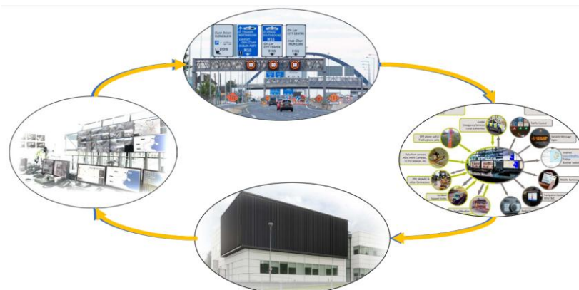
Figure B.24: NIMS in Ireland uses real-time data from multiple sources for dynamic traffic management on the M50 motorway (eMOS, 2024).
