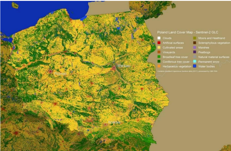
Figure B.5: Satellite land use and land cover data which are used with ML algorithms to inform changes in land use and environmental factors e.g. erosion or vegetation growth affecting road stability (ESA, 2024).
