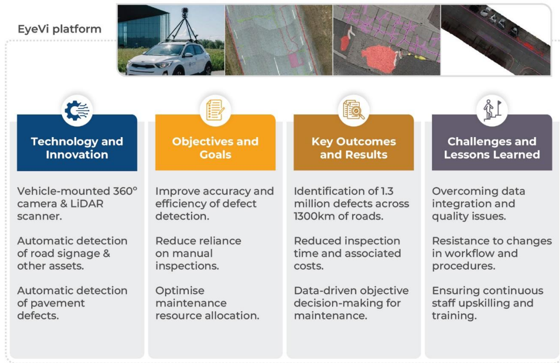
Figure 5.1: EyeVi platform - digitalisation of defects on Oslo's urban road network.
