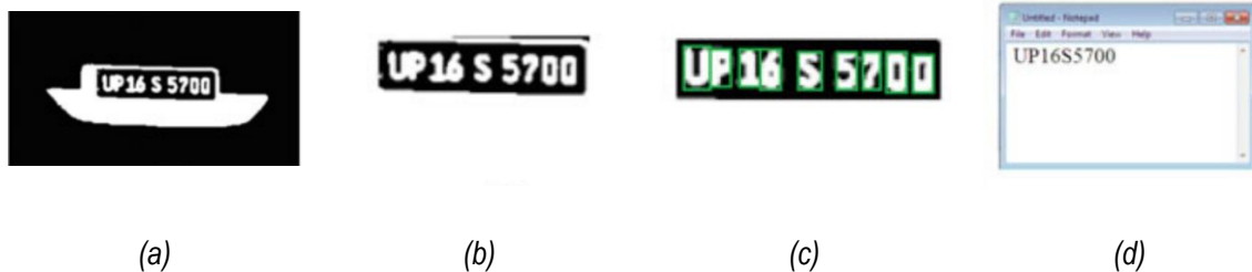
Figure B.31: (a) region of interest, (b) number of plate extraction, (c) character segmentation, (d) license plate recognition (Chavan et al., 2021).
