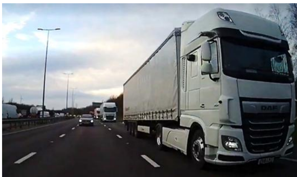
Figure 10. Platooning formation at 0.8 seconds time-headway during Safety Case validation on UK test track and on-road.
