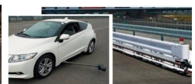
c. Power is fed by a pantograph sliding on a roadside rail 3)
