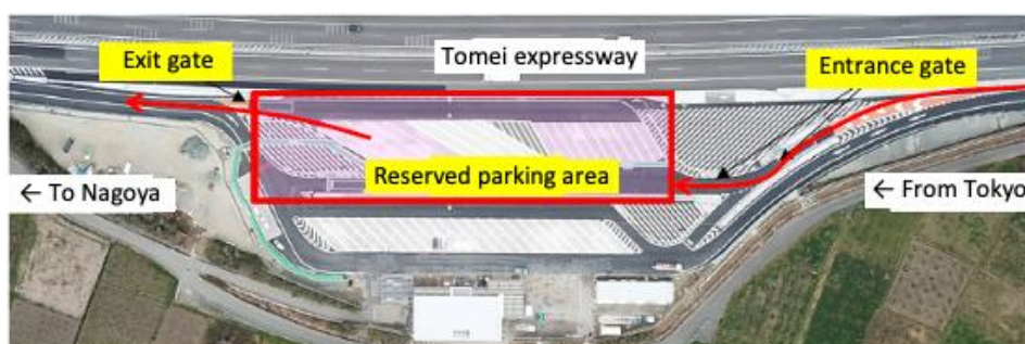
Figure 15. Layout of the parking spaces in Toyohashi Parking Area, where the Pricing Parking Reservation system is installed.
