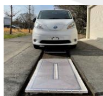
d. Power is fed through coils placed at the bottom of the vehicle 4)
