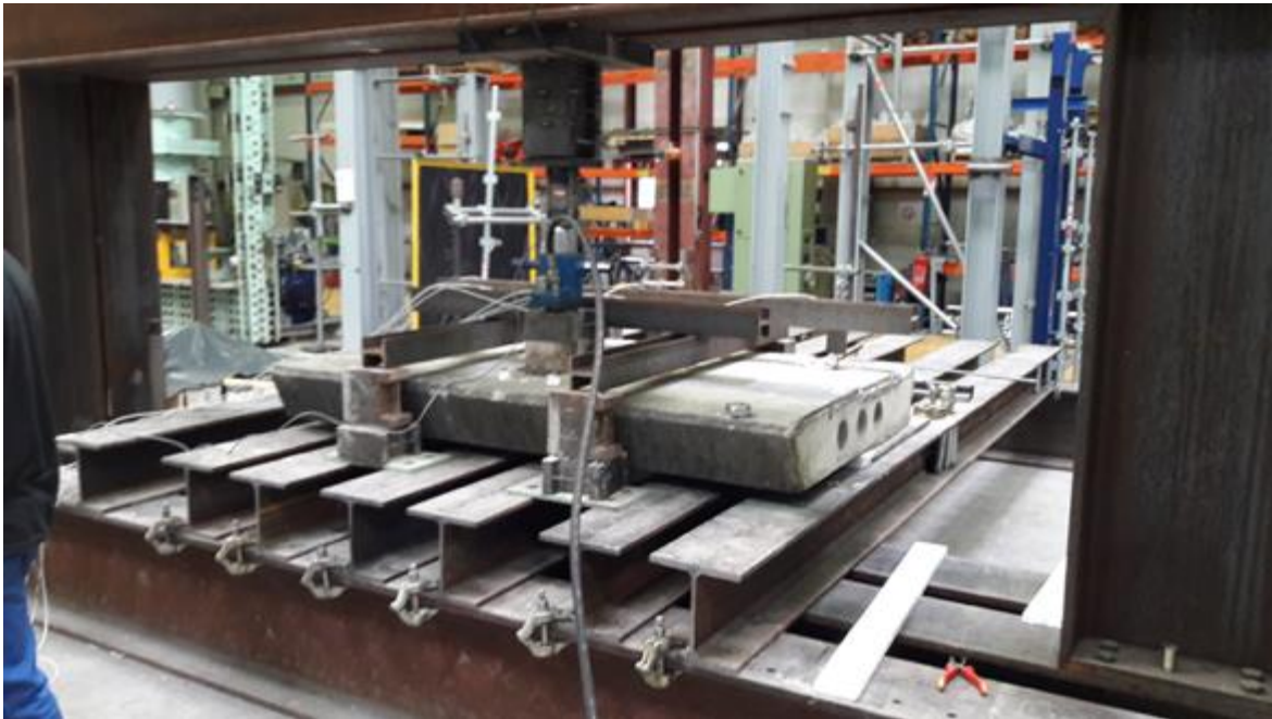
Figure 11: Scaled component experiments used to support the Cofiroute investigation a failed precast corbel sidewalk to deck slab connection at the Elancourt Structural Engineering Laboratory in Paris, France.
