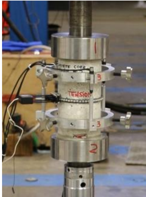
Figure 10: Concrete Elastic Modulus and Poisson's Ratio testing to support a rigorous structural analysis.
