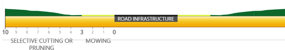
Figure 3.8 Road cross-section and distances for mowing and selective cutting or pruning in Portugal, [40].
