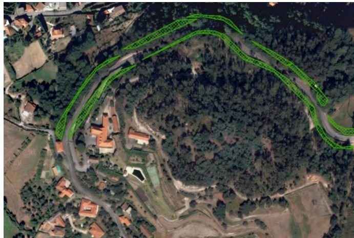
Figure 3.11 An example of a GIS processing for the identification of the roadside vegetation management areas under private property in Portugal, ©IP.
