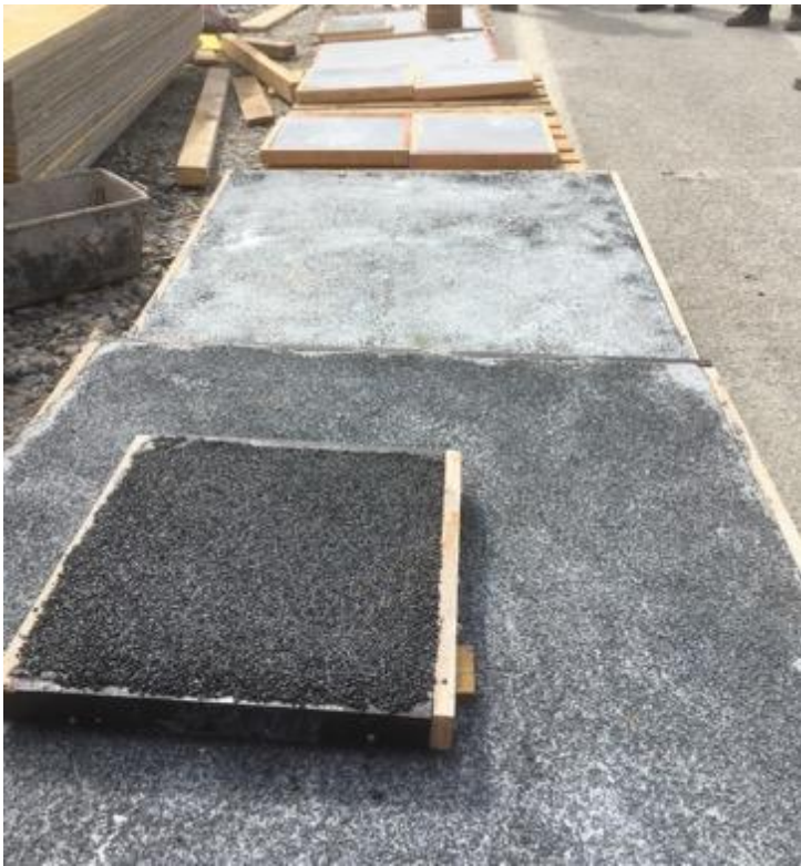
Other samples of the “splittmatrix” made with a different UHPC product.
