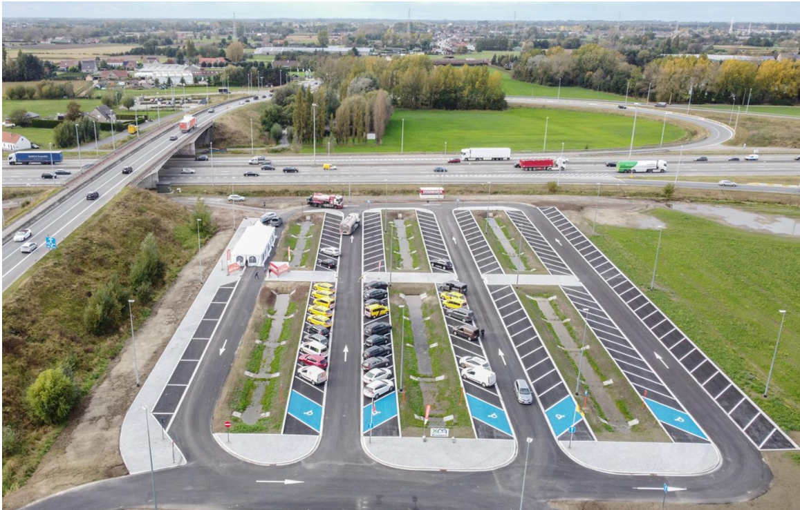
Figure 7.3.3-1: carpool parking in Kruisem with infiltration meadows, infiltration ditches and pervious bituminous pavements (photo: Agency for Roads and Traffic, Belgium)
