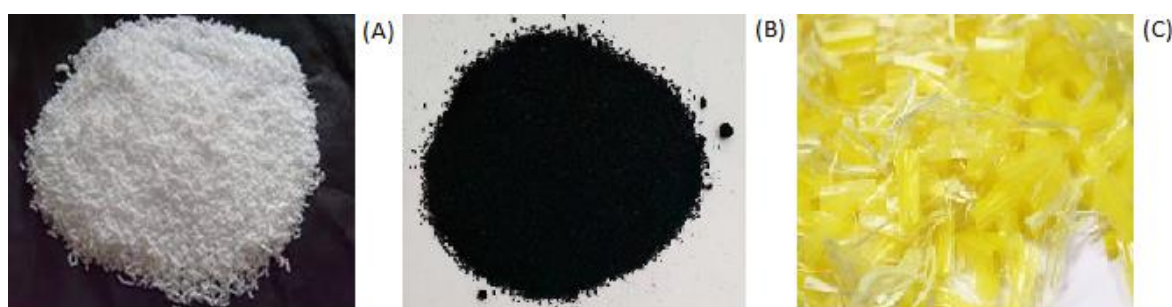
Figure 7.1.1-1: bitumen modifiers: SBS (A) crumb rubber (B) synthetic fibres (C) [7.1.1-2, 7.1.1-3]
