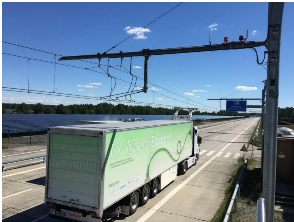
Figure 6: A Catenary Electric Road System
