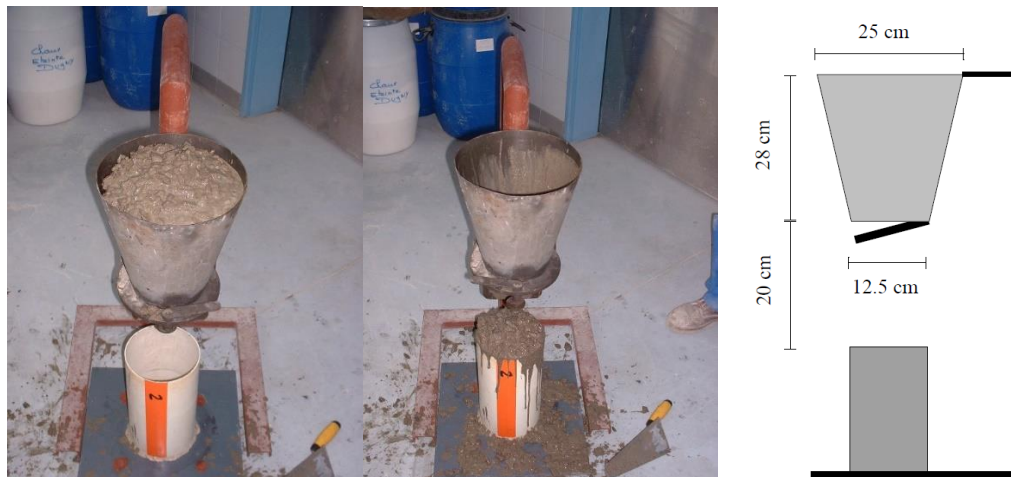
Figure 49: Measurement of the self compactability of the material by filling \varnothing 16\text{cm} \times 32\text{ cm} cylinders with the Glanville apparatus (from [2] and [3])
