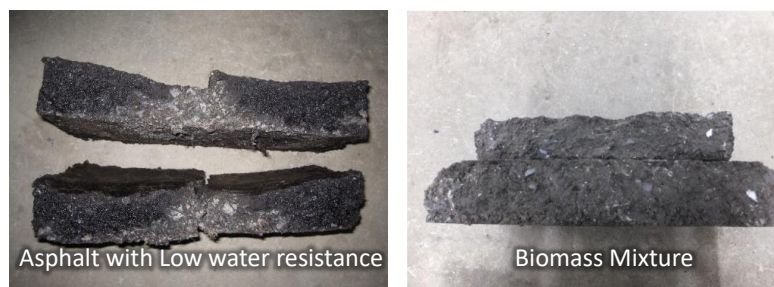
Figure 40: The result of immersed wheel tracking test
