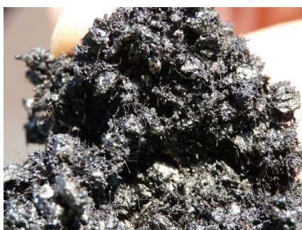
Figure 19: Aspect of microsurfacing with the addition of fibers
