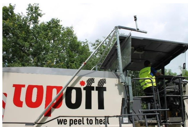
Figure 6: Milling machine with prism
