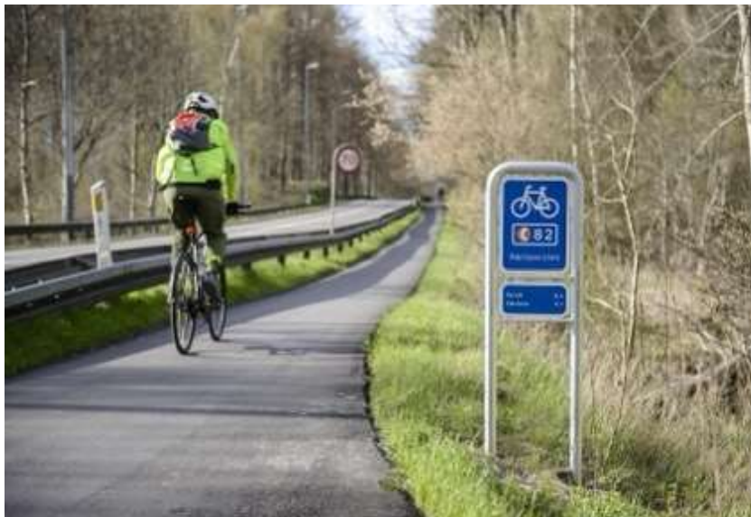
Danish cycle superhighway, with physical separation and clear route identification and destinations pointers.
