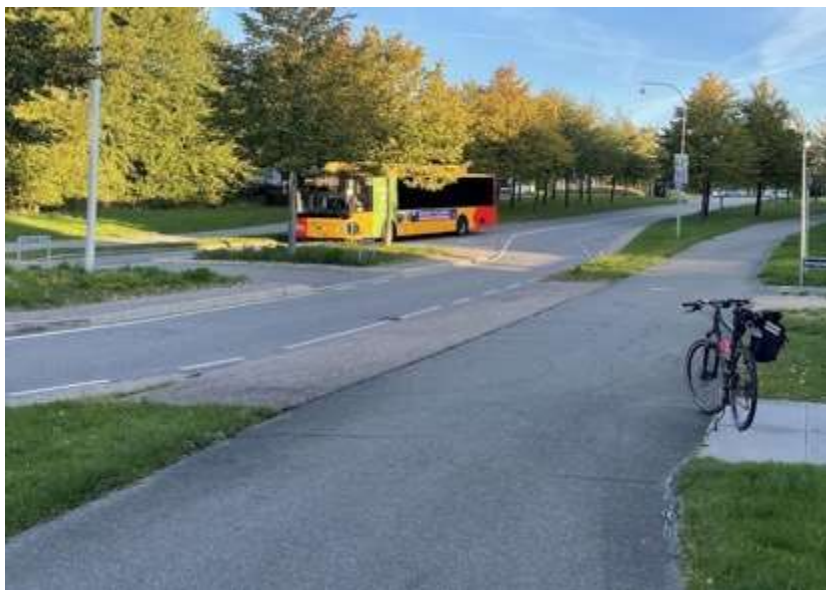
Cycling track separated by grass strip and curb.
