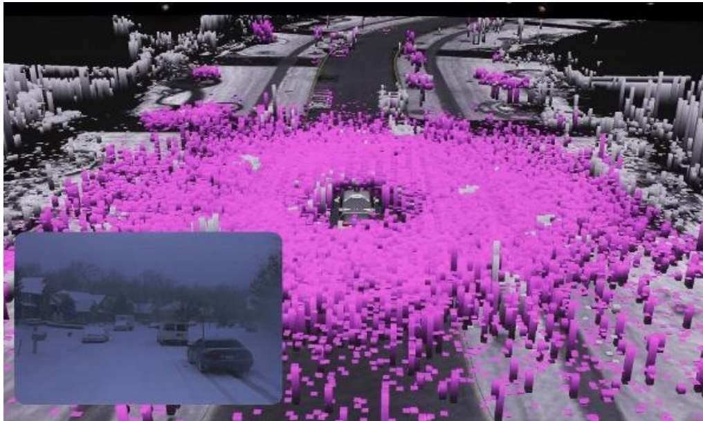
Figure 14: LIDAR rendering of a snowfall - numerous of purple cloud point (source: Waymo)
