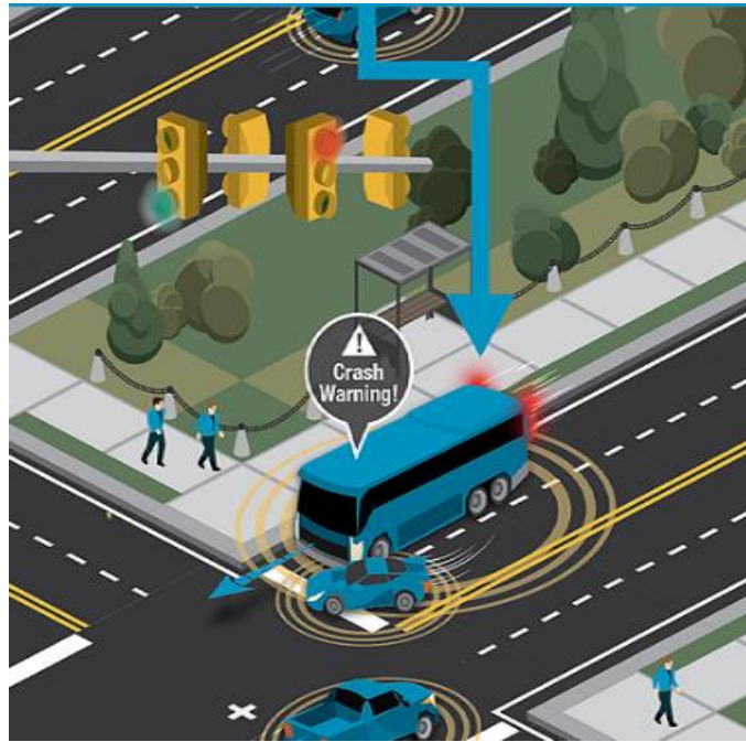
Figure 28: Vehicle Turning Right in Front of Bus Warning
