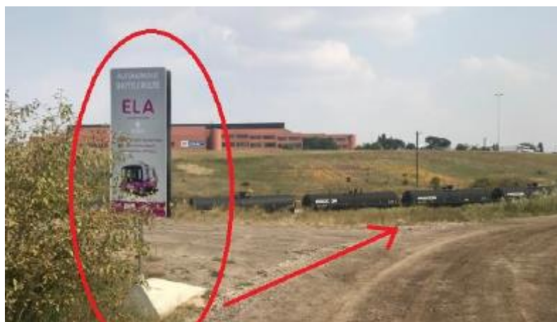
Figure 16: Example of foliage blocking a low-speed shuttle landmark [4]
