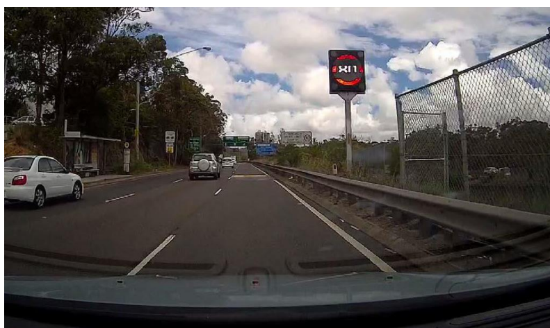
Figure 8: Examples of the effect of LED refresh rates - blackened sections.
