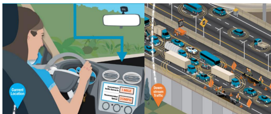
Figure 31: Queue Warning (Q-WARN)
