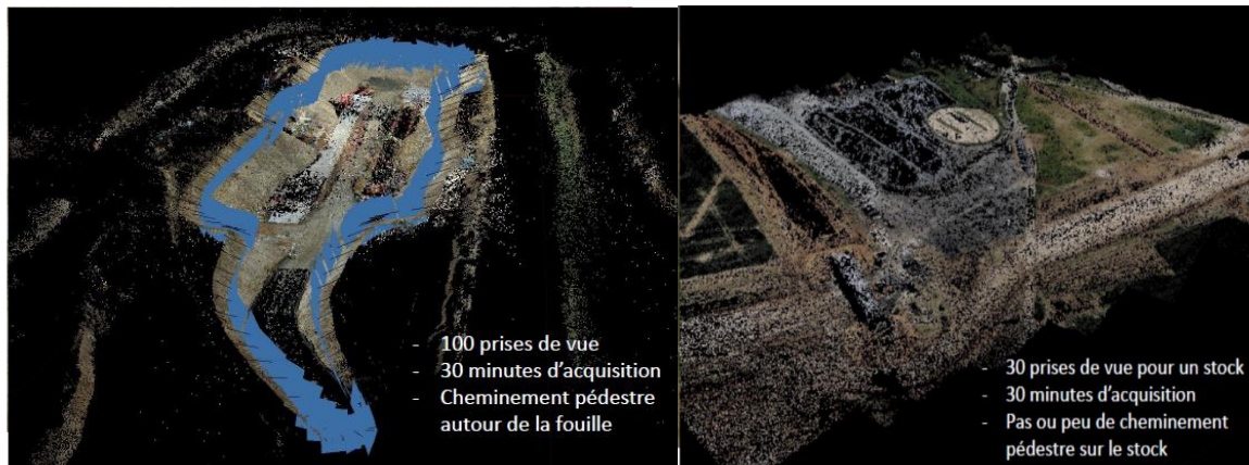
Figure 6: example of the result of a lidar acquisition
