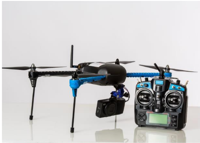
Figure 5: example of drone and on-board camera
