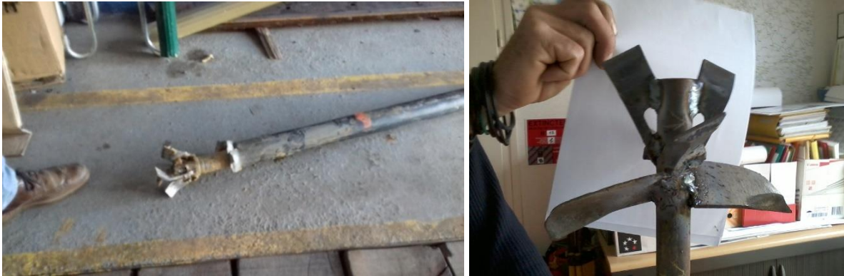
Figure 20: A specific tool has been adapted to incorporate lime into the soil with a vertical borehole
